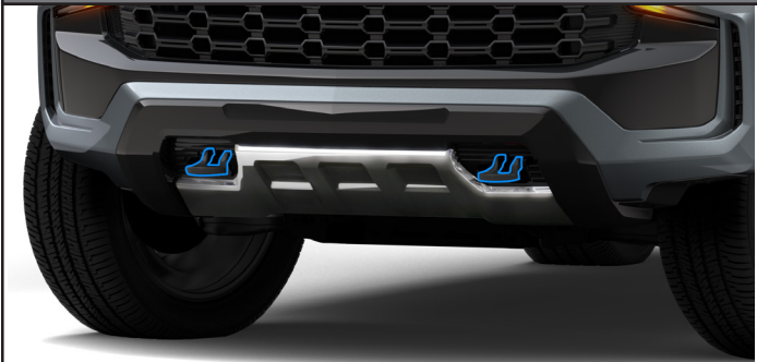
Two black front frame mounted. 1 NOTE: Front recovery hooks are for vehicle recovery only. To avoid the risk of injury, never use recovery hooks to tow a vehicle.
