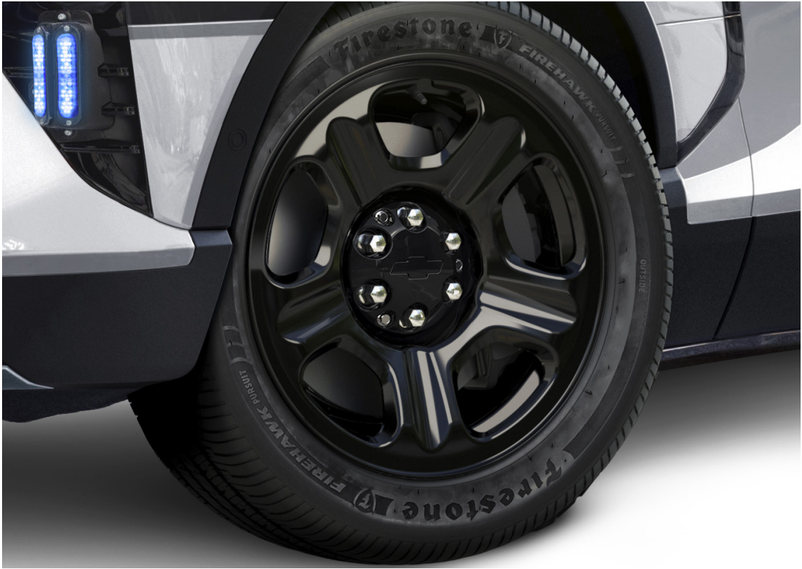
STANDARD HEAVY-DUTY STEEL WHEEL WITH FIRESTONE FIREHAWK PURSUIT TIRE
