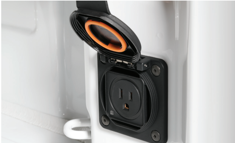
Standard 120-volt power outlet in bed
