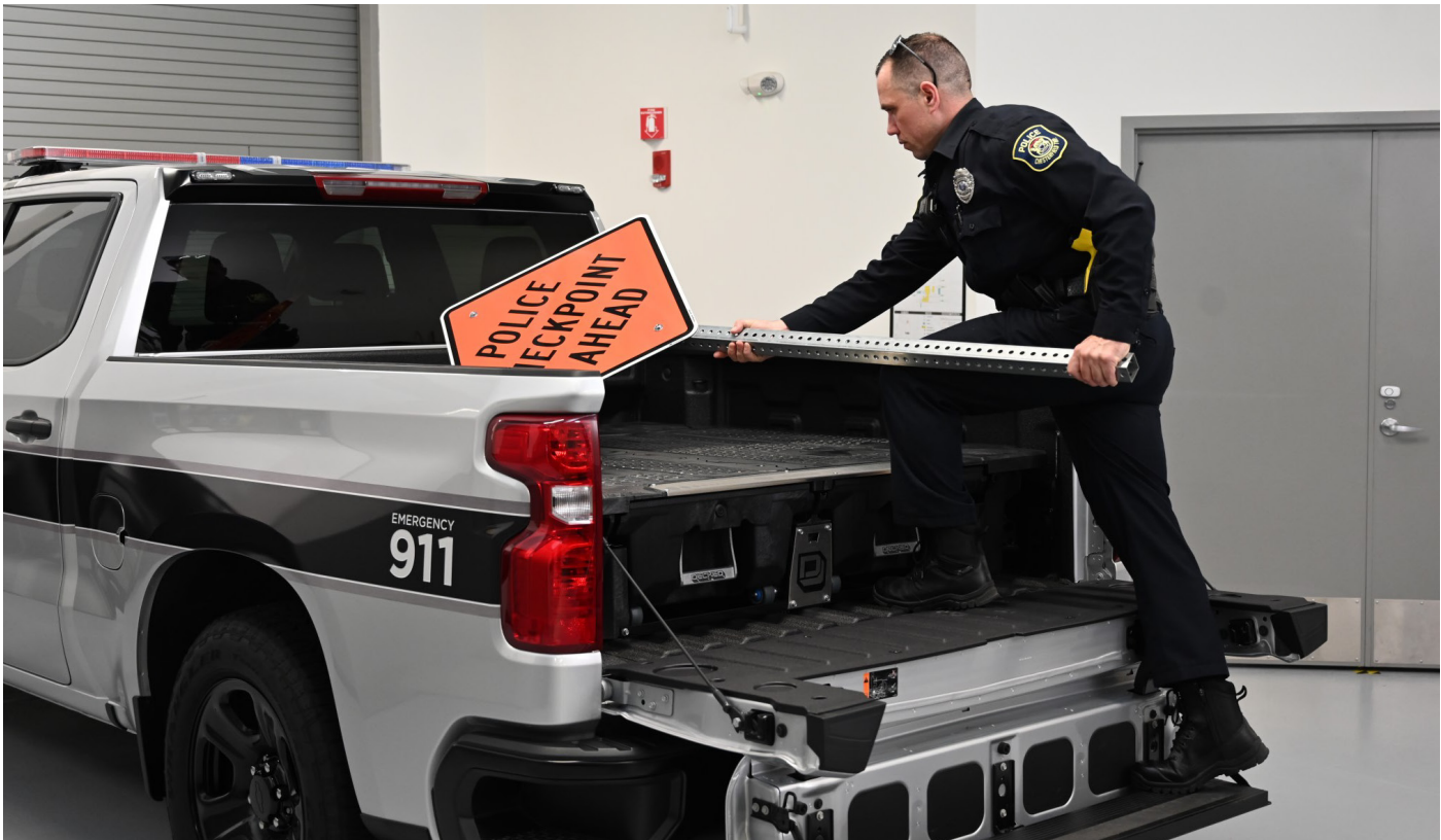
Six function gate (Primary, easy access, load stop, full width step, inner gate load stop, inner gate work surface)
