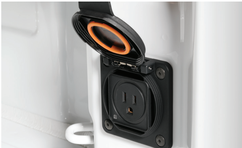
Standard 120-volt power outlet in bed
