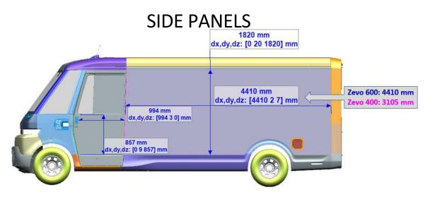
The only difference between BrightDrop 400 and BrightDrop 600 is the length of the cargo side panel & roof panel. Please see pic. The rest of the dimensions (front, side, & rear) are the same as BrightDrop 600.
