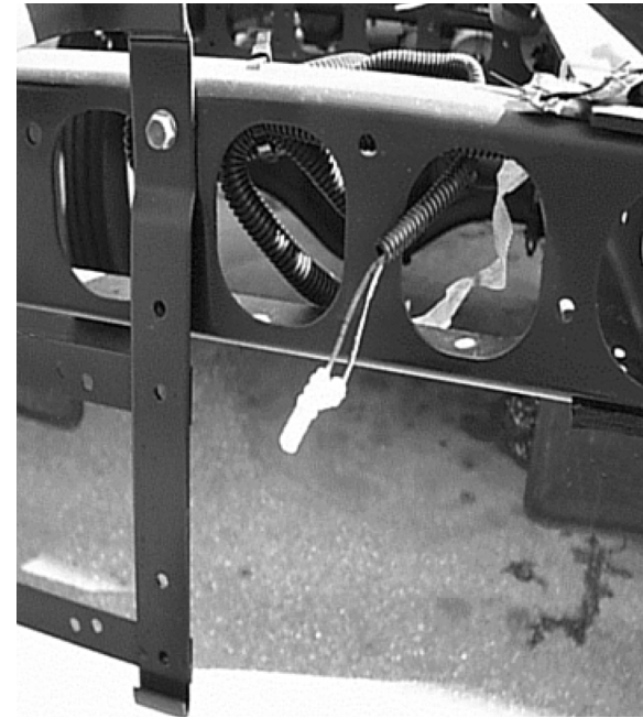
FRR Back-Up Alarm Wiring
